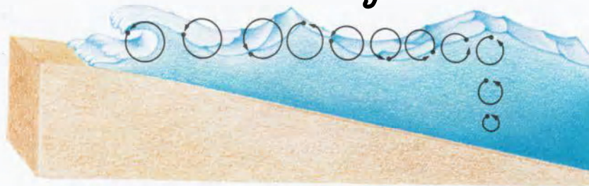
Left: Water particles on the ocean's surface move in a circle as a wave passes. Despite appearances, they are not carried along with the wave. Right: A breaking wave advances toward shore where it is met by the backwash from a previous wave (a-c). After the wave breaks and washes onto land (d-f), it also becomes backwash and the cycle repeats.
